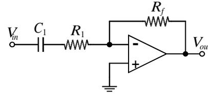
$$\frac{V_{out}}{V_{in}}(j\omega) = -\frac{Z_f}{Z_1} = \frac{-R_f}{R_1 + \frac{1}{j\omega C_1}} = \frac{-R_f}{R_1} \frac{j\omega C_1 R_1}{1 - j\frac{1}{\omega C_1 R_1}} = \frac{-R_f}{R_1} \frac{j\omega C_1 R_1}{1 - j\frac{f_L}{f}}$$
