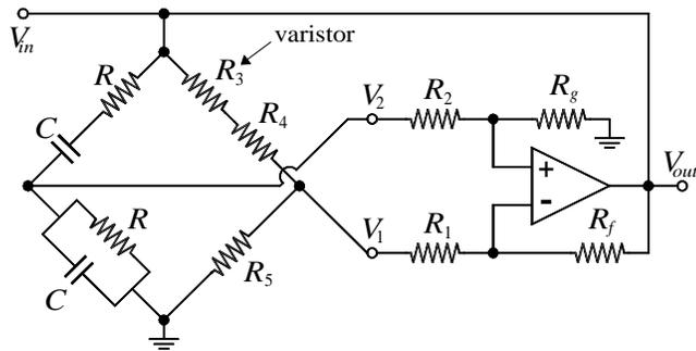
Find  $V_1$  and  $V_2$ :  $V_1 = V_{in} \frac{R_5}{R_3 + R_4 + R_5}$
