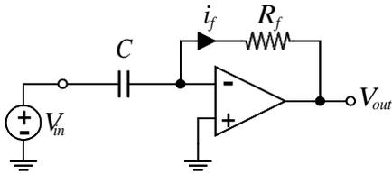
$$V_{out} = -i_f R_f = -R_f C \frac{dv_{in}}{dt} \quad f_C = \sqrt{f_B f_u}$$
