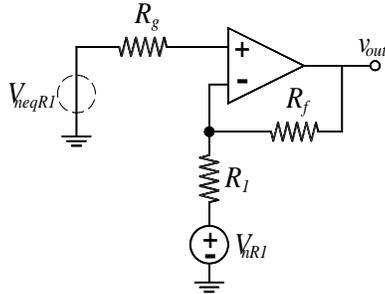
$$V_{neqR1} \frac{R_1 + R_f}{R_1} = V_{out} = -\frac{R_f}{R_1} V_{nR1}$$
