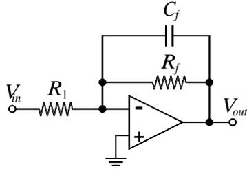
$$\frac{V_{out}}{V_{in}}(j\omega) = -\frac{Z_f}{Z_1} = -\frac{1}{j\omega C_f} \parallel R_f \Bigg| R_1 = \frac{-R_f}{R_1} \frac{1}{1 + j\omega C_f R_f}$$
