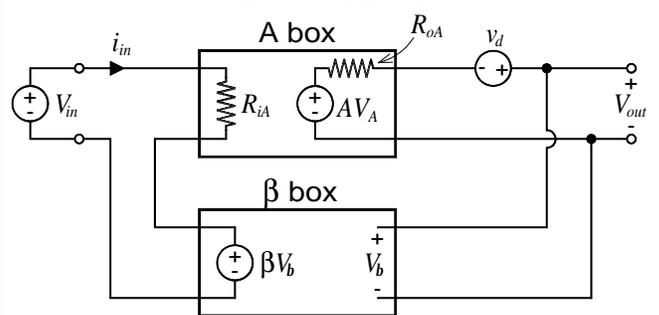
$$V_{out} = \frac{A}{1 + \beta A} V_{in} + \frac{1}{1 + \beta A} v_d$$
