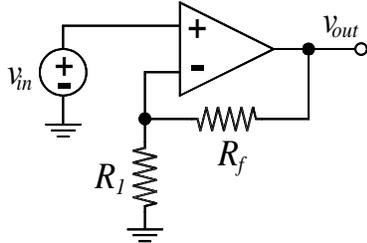
$$A_f = \frac{v_{out}}{v_{in}} = \frac{1}{\frac{1}{A} + \frac{R_1}{R_1 + R_f}}$$
