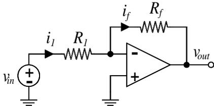
$$A_{f\infty} = \frac{v_{out}}{v_{in}} = -\frac{R_f}{R_1}$$
