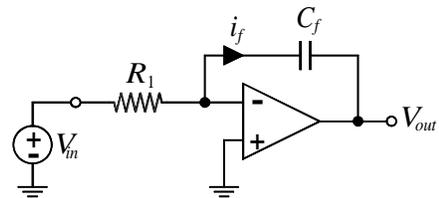
$$V_{out} = -\frac{1}{C_f} \int_0^t i_f dt = -\frac{1}{C_f} \int_0^t \frac{V_{in}}{R_1} dt = -\frac{1}{C_f R_1} \int_0^t V_{in} dt$$
