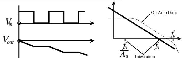
$$\text{Gain: } \frac{V_{out}}{V_{in}}(j\omega) = -\frac{Z_C}{R_1} = \frac{-1/j\omega C}{R_1} = j \frac{1}{2\pi f C R_1}$$
