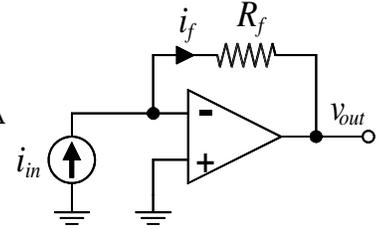
$z_{in}$  is typically less than  $1 \Omega$
