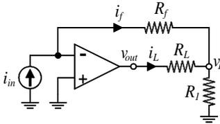
$A_{f\infty} = \frac{i_L}{i_{in}} = -\frac{R_1 + R_f}{R_1} \text{ A/A}$        | <p style="text-align: center;"><b>Transconductance</b></p>
