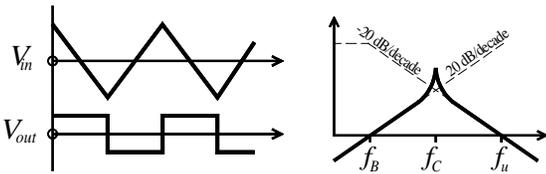
$$\text{Gain: } \frac{V_{out}}{V_{in}}(j\omega) = -\frac{Z_f}{Z_1} = -\frac{R_f}{1} \frac{1}{j\omega C} = -j2\pi f C R_f$$
