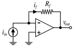
$A_{f\infty} = \frac{v_{out}}{i_{in}} = -R_f \text{ V/A}$         |
