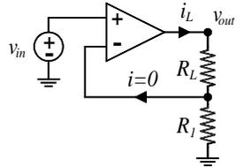
$A_{f\infty} = \frac{i_L}{v_{in}} = \frac{1}{R_1} \text{ A/V}$ |
