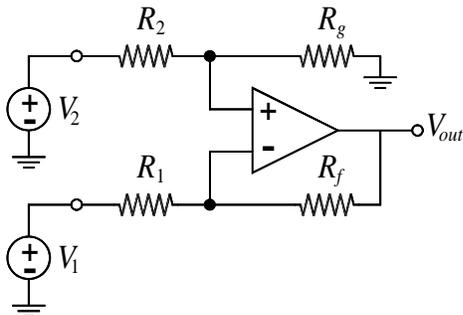
By superposition, the output is  $V_{out\ V1} + V_{out\ V2}$ .
