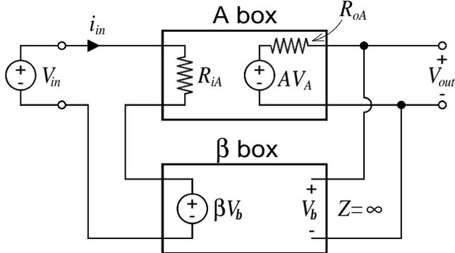
$$A_f = \frac{v_{out}}{v_{in}} = \frac{A}{1 + \beta A}$$
