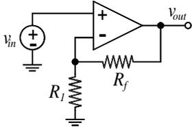
$A_{f\infty} = \frac{v_{out}}{v_{in}} = \frac{R_1 + R_f}{R_1} \text{ V/V}$ | <p style="text-align: center;"><b>Transresistance</b></p>
