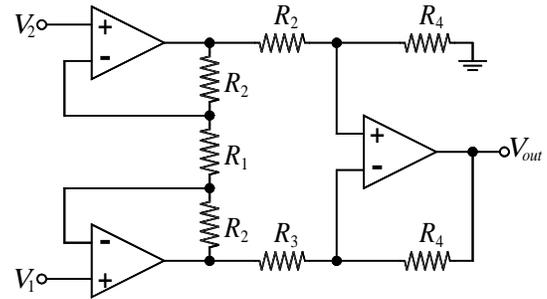
$$A_{diff} = \frac{R_4}{R_3} \left( 1 + 2 \frac{R_2}{R_1} \right)$$
