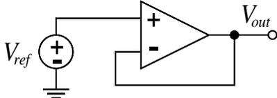
If  $A$  is very large then  $V_{out} = V_{ref}$
