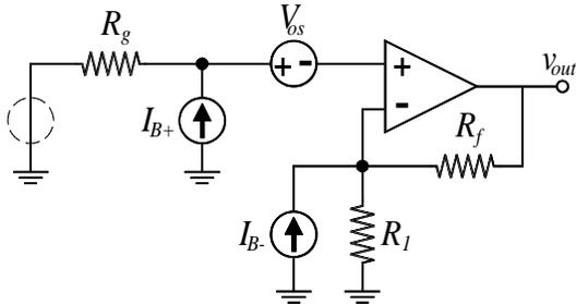
The offset voltage is equal to the voltage at the positive input multiplied by the gain, added to the voltage at the output resulting from current  $I_{B-}$ . For the **worst case offset** for this amplifier, let  $I_{B+} = I_{B-} + I_O$ .
