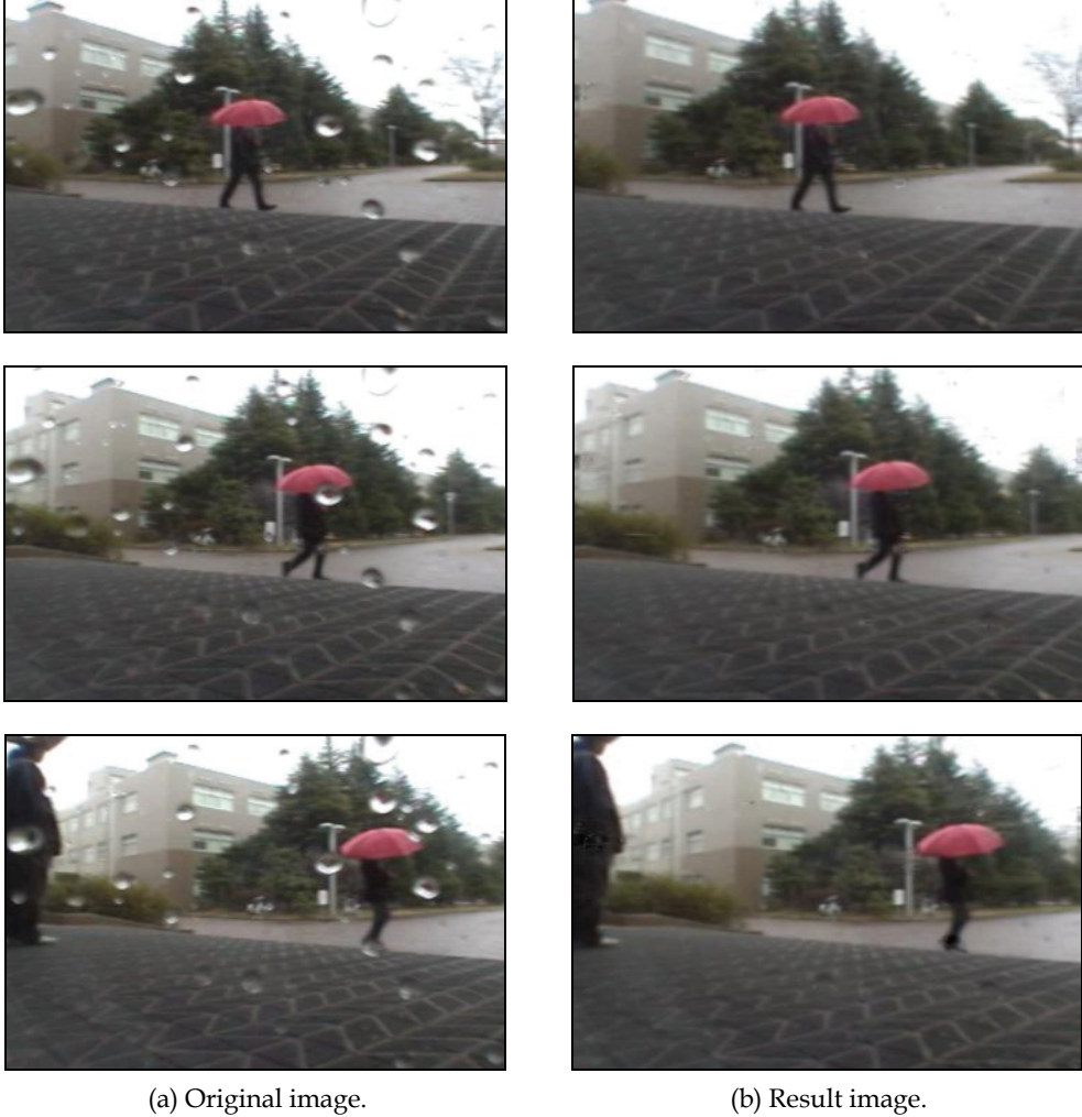
Fig. 12. Results of noise removal (waterdrop).
