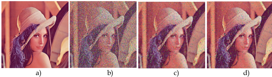
Fig. 9. Subjective visual qualities of restored color image “Lena”, a) Original test image “Lena”, b) Input noisy image with 20% of impulsive noise, c) MAMNFE filtering image, and d) Proposed VMMKNN (S) filtered image.
