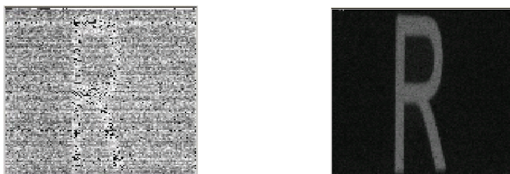
Fig. 17. Images with FPN (left) and with removed FPN (right)
