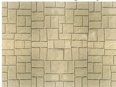
d. brick surface 3D height map extracted from image processing
