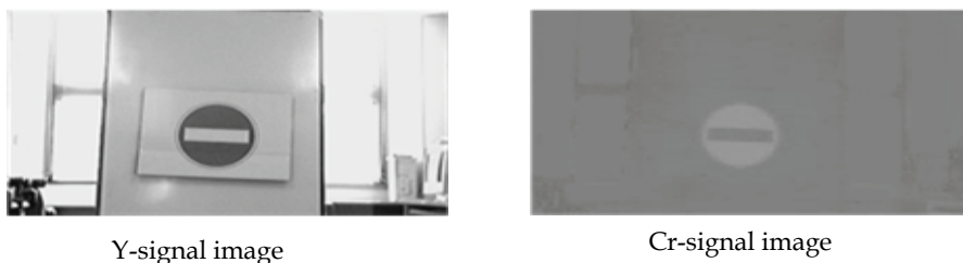
Fig. 5. Image YCrCb signals, converted from RGB signals.
